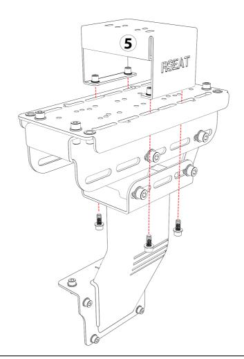
**Thrustmaster TSS Sequential Shifter Sparco Mod,** DSD Pro Pro Sequential Shifter - Install the shifter on top assembly (1) WWW.rseat.net with no adapter plate. Use 4xM6x20mm screws provided.
