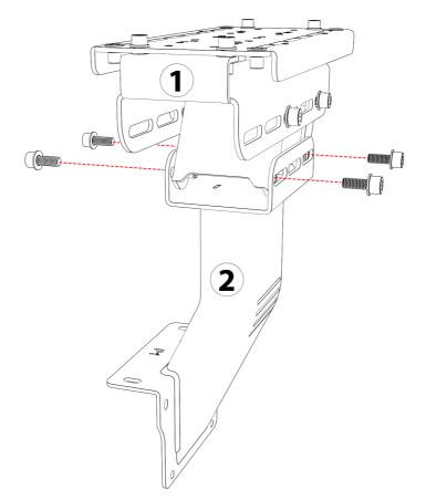
Install P1 Shifter Handbrake Upgrade kit on **Left or Right** side of P1 chassis.
