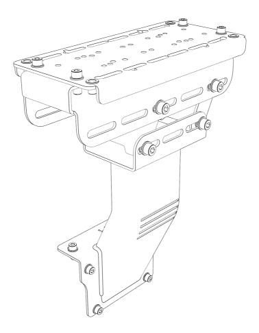
**Handbrake Support** - Install Thrustmaster TSS handbrake Sparco mod, Fanatec Clubsport handbrake on adapter plate (4), use 4xM6x20 screws. Next install the adapter plate on P1 shifter/handbrake top assembly (1) use 4xM8x20mm screws and 6mm Hex Key
