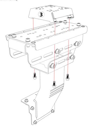
**Thrustmaster/Logitech Shifters** - Install the Thrustmaster/Logitech Shifter on adapter plate (5), use 2xM6x20 screws provided. Next install the adapter plate on P1 shifter/handbrake top assembly (1) use 4xM8x20mm screws and 6mm Hex Key
