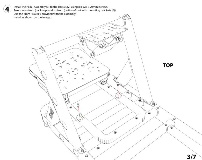
Install the Pedal Assembly mounting brackets (6) to the chassis (2) (red lines) using  $4 \times (M8 \times 20 \text{mm})$  screws. Fix the Pedal Assembly (3) to mounting brackets (6) (blue lines) with  $2 \times (M8 \times 20 \text{mm})$  screws. Use the 6mm HEX Key
