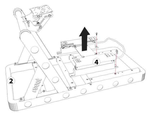
Install the 4 x foot steps (M8 thread) to B1 chassis (2). Use 10mm wrench to adjust chassis level to the floor.
