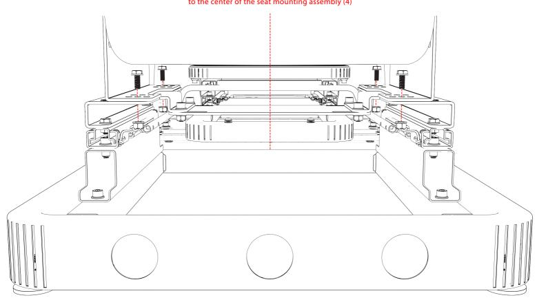
Now adjust the seat position to seat mounting bracket (5) - (height, tilt) and tight the seat using the 6mm HEX Key provided with the assembly.
