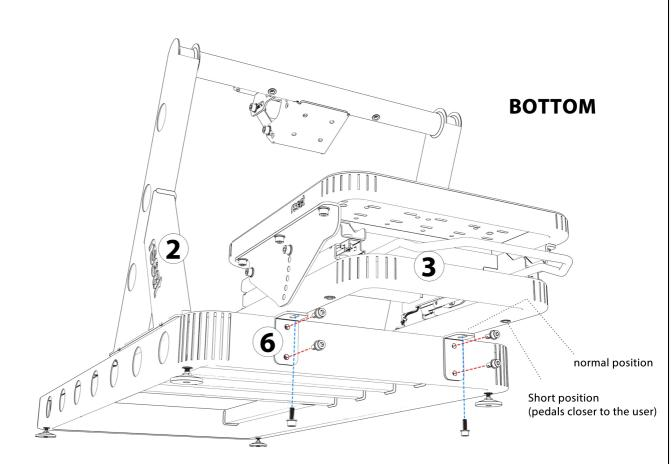
Slide the Pedal Assembly aluminum cover under pedal mounting plate and secure with  $4\,x$  (M8 x 20mm) screws. Use the 6mm HEX Key
