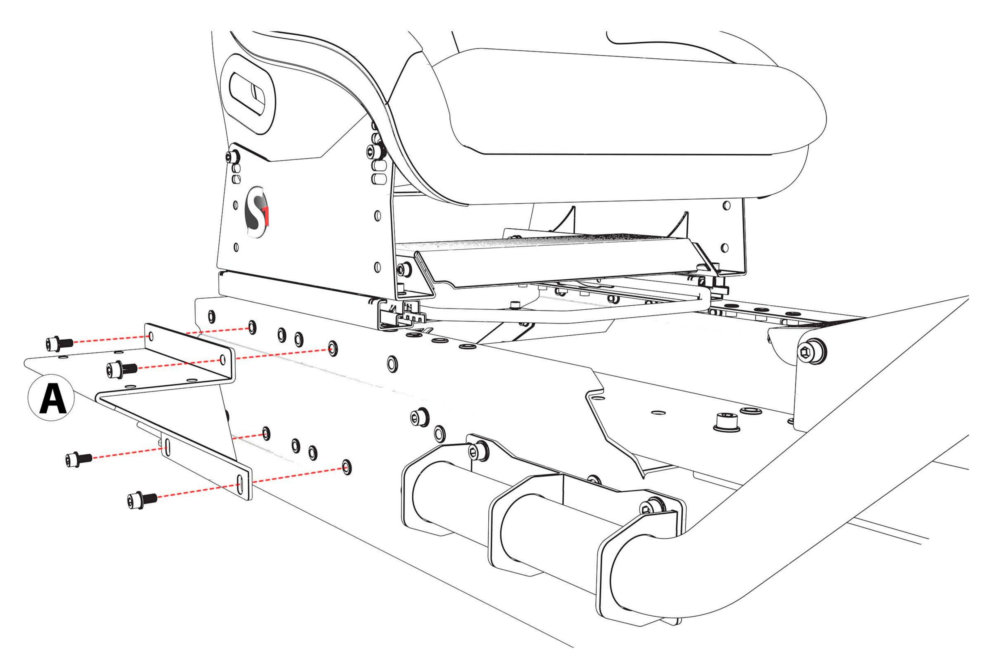
Install the Main Support (A) to Main Support (B) using 4 x (M8x20mm) allen head bolts provided with the assembly instruction (F). Use the 6mm HEX Key . Perform same installation on the left side of the S1 chassis. Install as shown on the image below.
