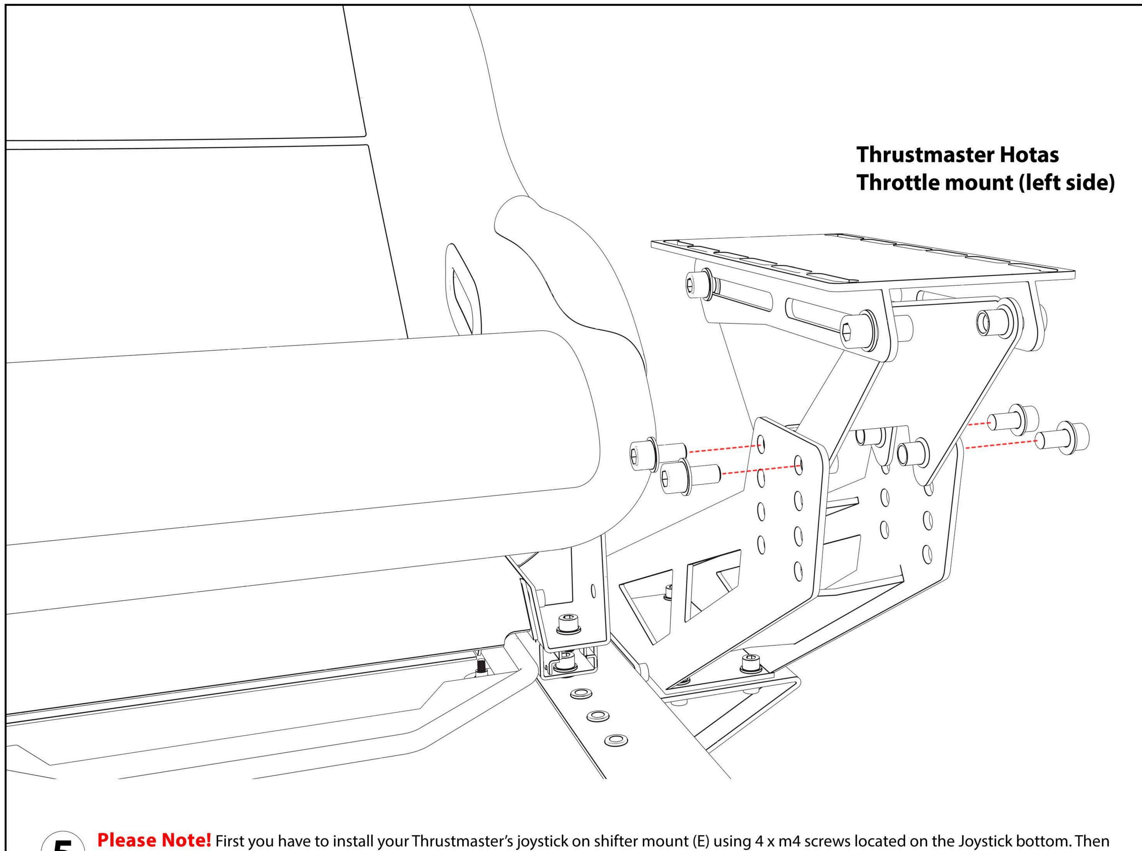
Please Note! First you have to install your Thrustmaster's joystick on shifter mount (E) using 4 x m4 screws located on the Joystick bottom. Then install (E) on sub assembly (C) using 4 x (M8x20mm) bolts. Use 6mm Hex key. Install as shown on the images below.
