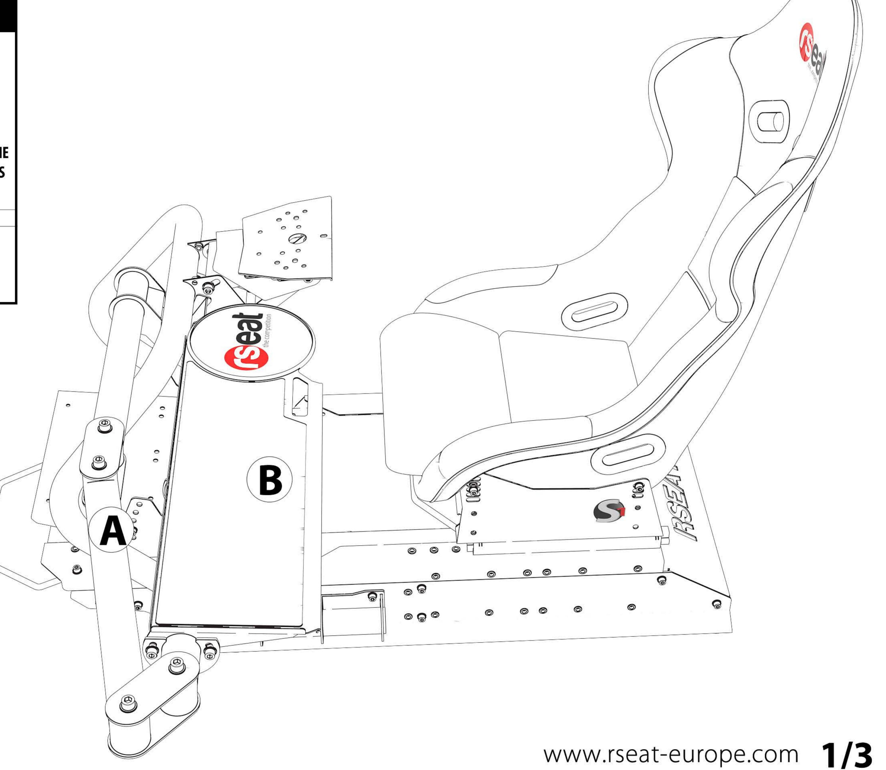
Install the Keyboard/Mouse tray adjustable arm (A) using 1 x (M10x45mm) screw to the S1 chassis. Use the 8mm HEX Key provided witht the package(C) Install as shown on the images below.
