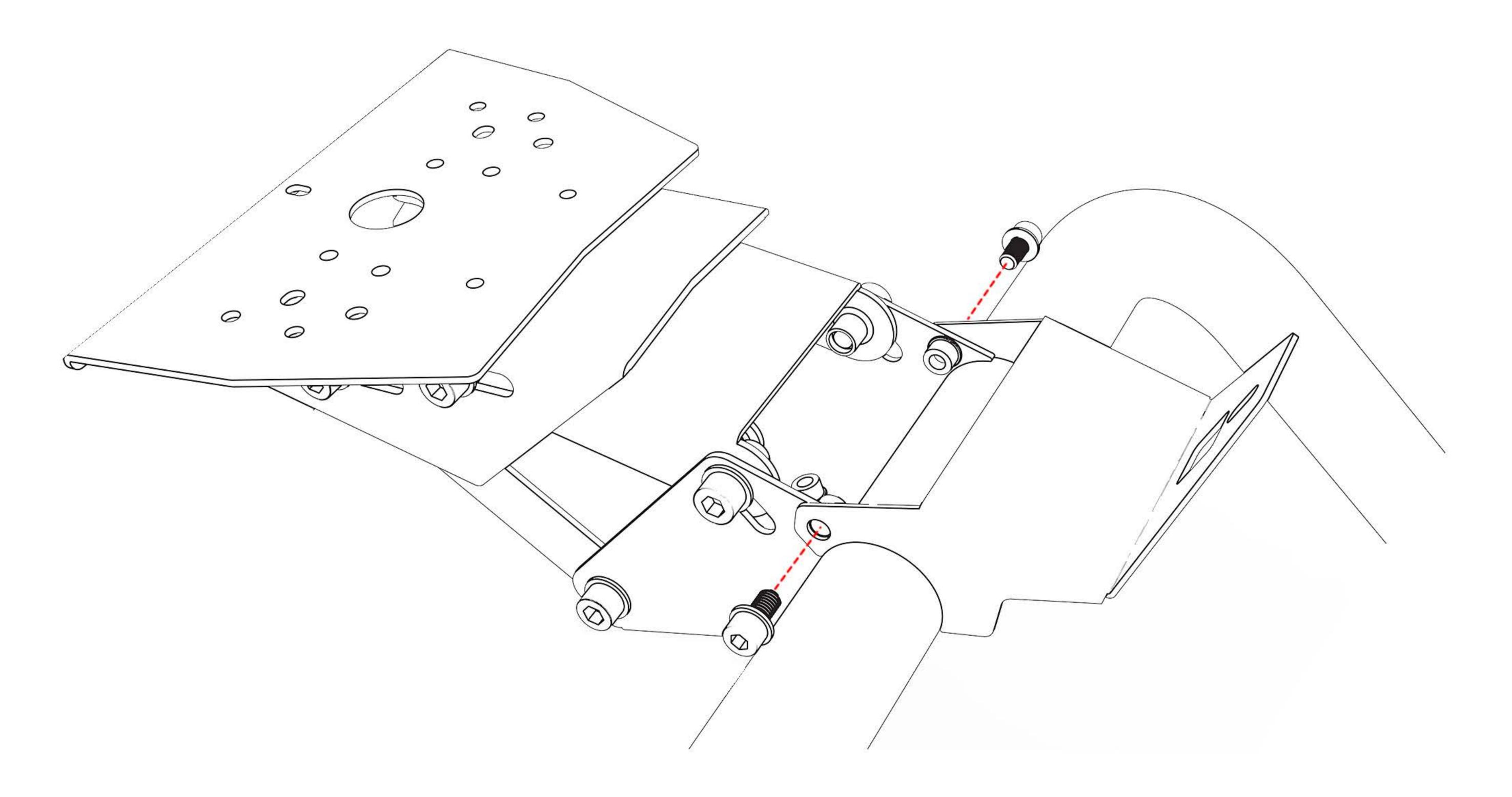
Install the Rear-left and Rear-right speaker mounts (C,D) using 1 x (M8x20mm hex head bolt) screws for each side. Use the 13 mm wrench provided witht the package(F) Install as shown on the image below.
